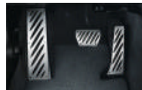
Aluminium pedal pads
