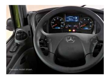
To give you both comfort and peace of mind out on the road, we've included just about everything you could possibly need for general distribution in the new Atego. The multifunction steering wheel, pneumatically adjustable for height and reach, has buttons to control the radio, telephone and driver information system.
