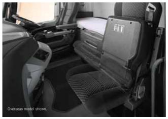
**Distribution:** The dimensions of the standard "Distribution" cockpit are such that it enables extremely convenient through-cab access whilst still featuring plenty of handy stowage space. A centre seat can be ordered as an option.
