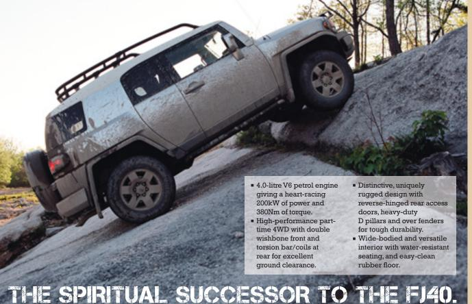
toughest terrain. Under the welded steel body are adaptations of the same tough and tested systems found on the LandCruiser Prado. A solid rear axle with a five-link coil-spring system combined with serious wheel articulation all add up to genuine off-road
