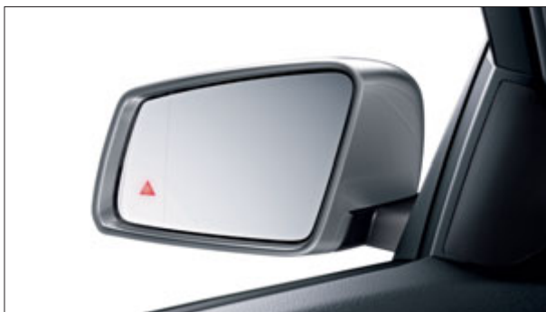
Blind Spot Assist can warn of potential dangers acoustically and via a red warning triangle in the exterior mirror
