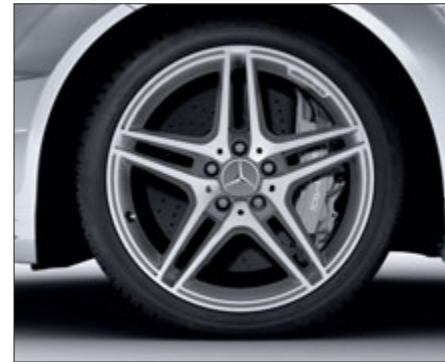
5-twin-spoke AMG light-alloy wheels, painted titanium grey with a high-sheen finish, with 235/40 R 18 front tyres and 255/35 R 18 rear tyres (standard for C 63 AMG, Code 795)
