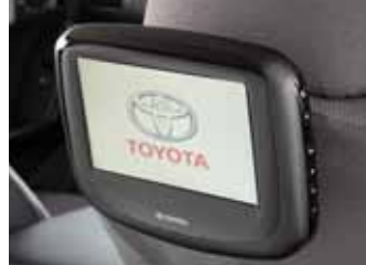
Rear Seat Entertainment Master unit reads CD, DVD, SD Card and USB 3 thumbdrive. Only applicable to KX-R and KX-S models.
