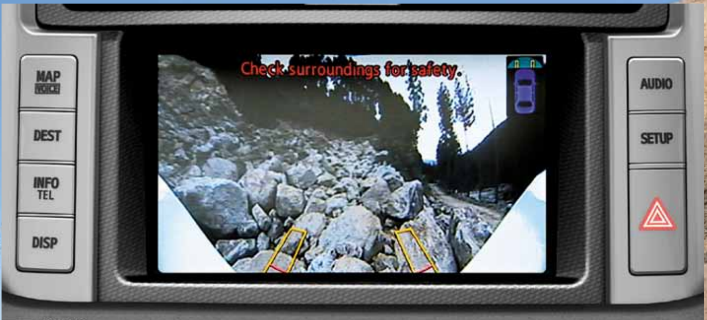
Multi-Terrain Monitor Camera View &amp; Steering Angle Display
