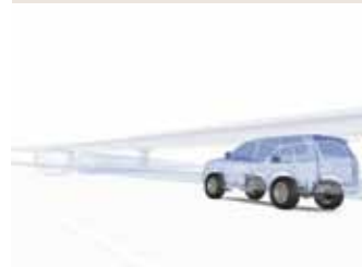
A. While on cruise control, millimetre-wave radar constantly confirms no obstacles are in the path of the vehicle.
