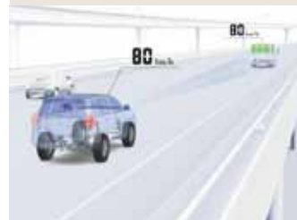
C. The system will maintain a constant distance from the vehicle in front based on your choice of three distance settings.
