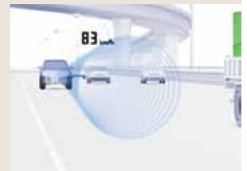
D. Once the path is clear the Radar Cruise Control System 1,2 will accelerate back to the predetermined speed setting.
