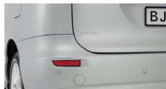
Park Assist 3 Reverse parking sensor-four-head kit (Shown on GLi. Available on all GLi models)
