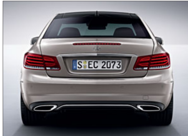
The Exterior Sports package with twin-pipe exhaust system featuring trapezoidal tailpipe trims in polished stainless steel attached to the bumper.
