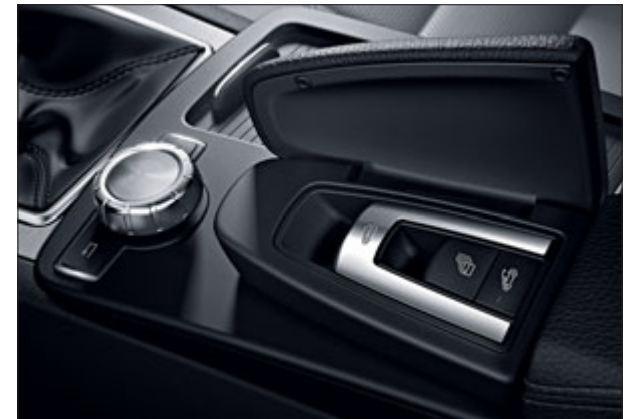
Soft-top operating switch (for Cabriolet only).
