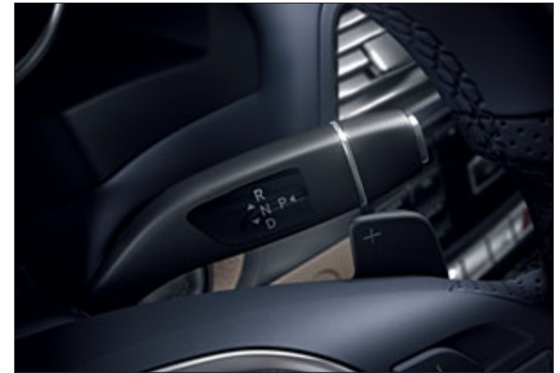
DIRECT SELECT lever and steering-wheel gearshift paddles.
