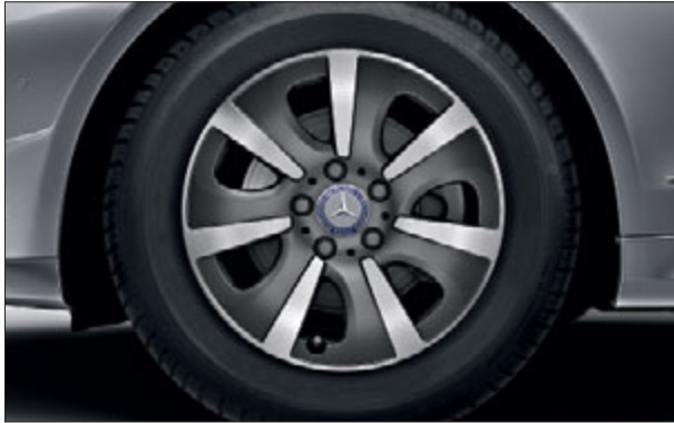
7-spoke aero-design light-alloy wheels with 205/55 R 16 tyres (no-cost option for all 4-cylinder models, Code 34R; only available for Coupé).
