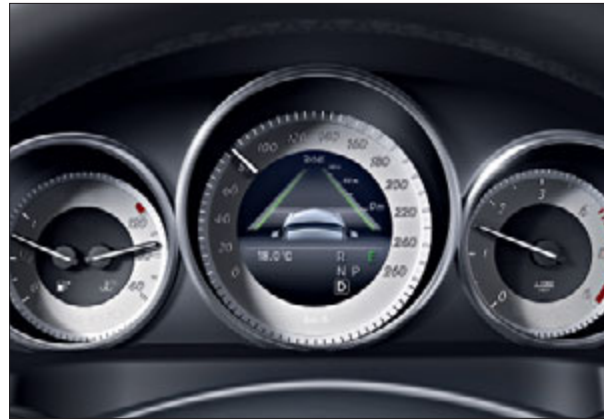
COLLISION PREVENTION ASSIST display in the 3-tube instrument cluster.
