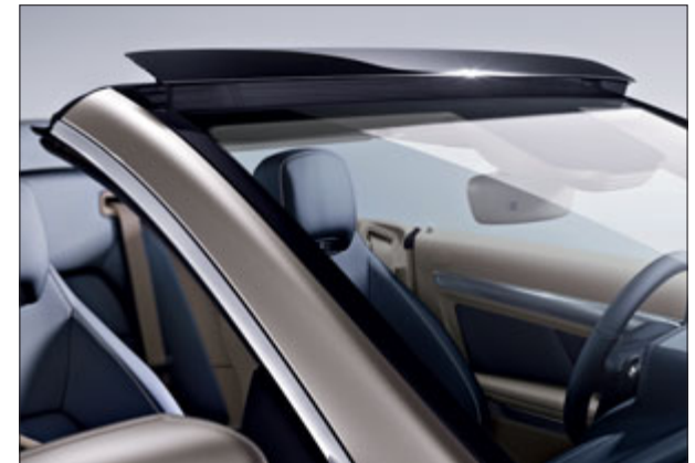
AIRCAP with electrical air deflector module (for Cabriolet only).
