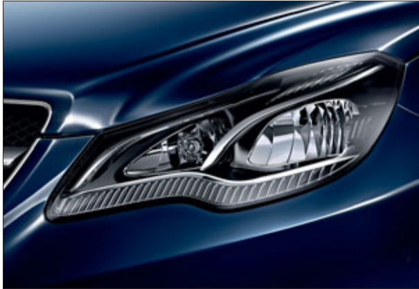
LED headlamps with LED main headlamps and LED daytime running lamps.
