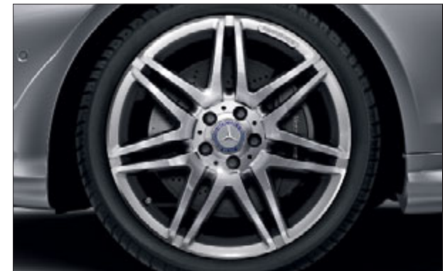
AMG 7-twin-spoke light-alloy wheels with high-shine finish, with 235/35 R 19 front tyres and 255/30 R 19 rear tyres (optional, Code 770).
