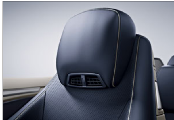
AIRSCARF with discreetly positioned nozzles (for Cabriolet only).
