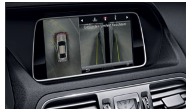
During parking, the COMAND Online central display shows the area around the car.
