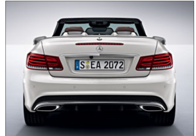
The AMG Sports package includes a twin-pipe exhaust system featuring trapezoidal tailpipe trims in polished stainless steel attached to the bumper.
