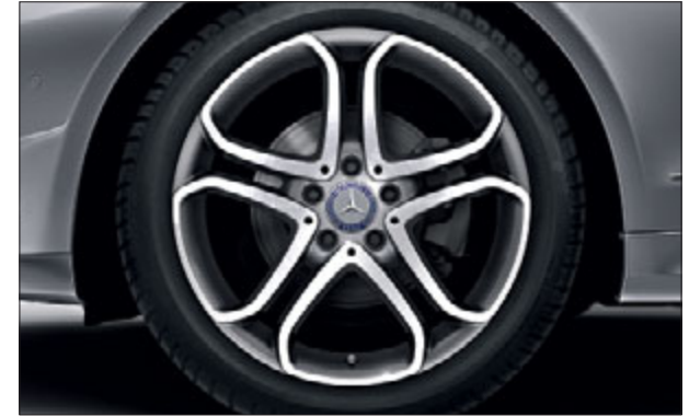
5-twin-spoke light-alloy wheels with 235/40 R 18 front tyres and 255/35 R 18 rear tyres (optional, Code R71, standard for 8-cylinder models, part of Exterior Sports package).
