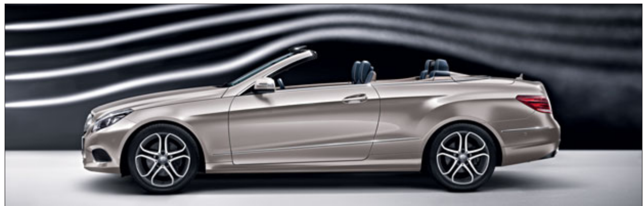
Simply ingenious: AIRCAP diverts the airflow above the heads of all four occupants.
