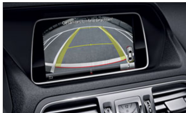
The reversing camera helps the driver with reversing by displaying static and dynamic guide lines.
