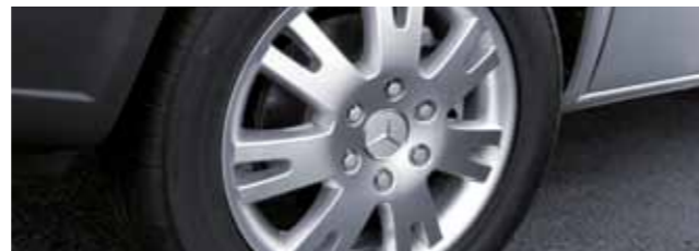
43.2cm (17") light alloy wheel B6 656 0390* 7 twin-spoke wheel in high-quality aluminium, with brilliant silver paint finish. Wheel size: 6.5 J x 17 ET 62 Tyre size: 235/60 R17 C
