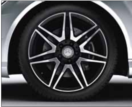
7-twin-spoke AMG light-alloy wheels, painted in high-gloss black with a high-sheen finish, with 225/40 R 18 front tyres and 255/35 R 18 rear tyres, (standard for AMG Plus Sports package and Sport models, Code 760).
