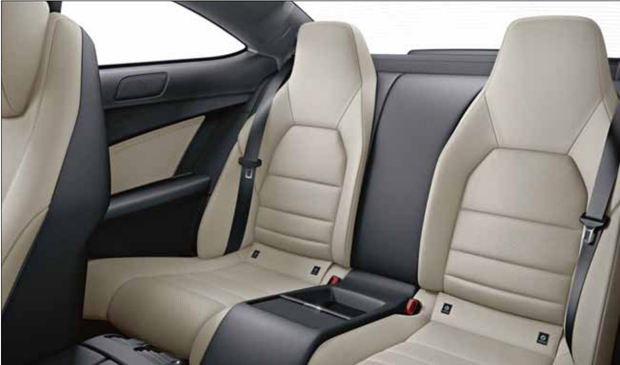
Sheer comfort: it's easy for rear passengers to get into the car thanks to the EASY-ENTRY system, which shifts the front seats fully forwards in one simple move.
