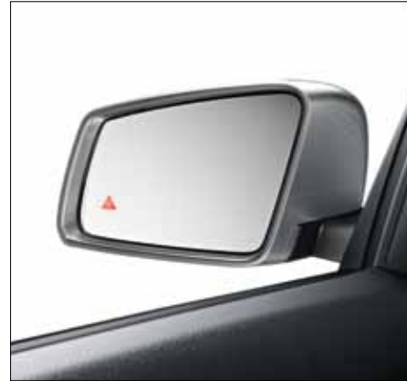
Blind Spot Assist monitors the blind spot and is able to warn of dangerous lane-changing manoeuvres.
