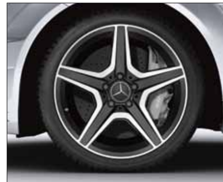
5-spoke AMG light-alloy wheels, painted in matt black with a high-sheen finish, with 235/40 R 18 front tyres and 255/35 R 18 rear tyres (optional for C 63 AMG, Code 609).
