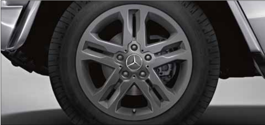
5-twin-spoke light-alloy wheels with 265/60 R 18 tyres, painted titanium grey (optional, only for Sports package, Code RM9).
