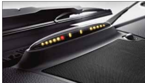
The PARKTRONIC LEDs indicate the distance to the obstacle.
