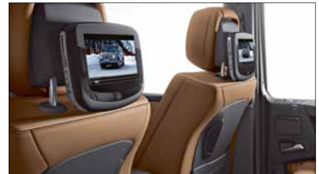
The two displays for the Rear Seat Entertainment System mounted on the front-seat head restraints.
