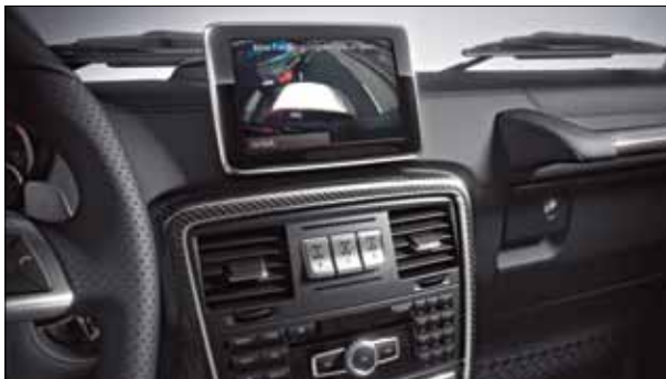
The reversing camera shows the area behind the vehicle during parking.
