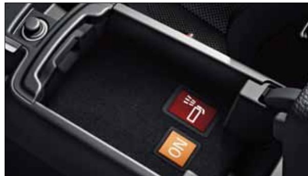
The fire extinguishing system, which can be deployed manually or automatically, can stop fire from breaking out in the interior.
