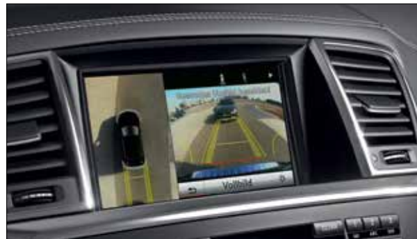
The 360° camera produces an image of the M-Class and its immediate surroundings from a bird's-eye view.
