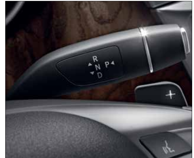
Transmission control with the DIRECT SELECT lever on the steering wheel. The driver can intervene manually in the gear selection process by using the shift paddles on the steering wheel.
