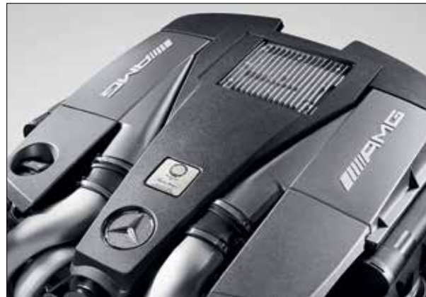
AMG engine cover in carbon fibre.
