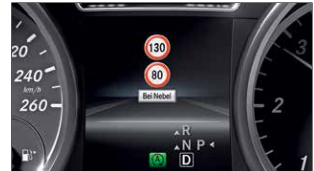
The information from Speed Limit Assist is shown both in the instrument cluster and in the COMAND Online central display.
