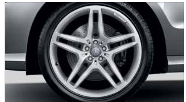
AMG 5-twin-spoke light-alloy wheels with 265/40 R 21 tyres, with a high-shine finish (optional).
