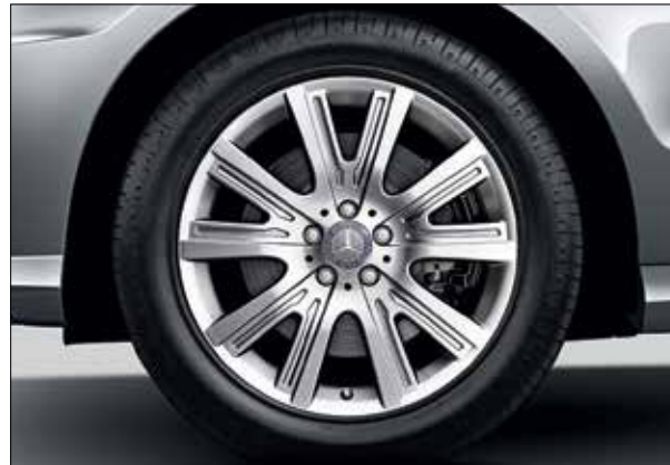
5-twin-spoke light-alloy wheels with 255/50 R 19 tyres.
