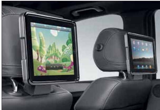
iPad® Rear Integration Plus makes all the functions of the iPad® available in the M-Class.
