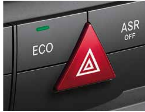
ECO Start/Stop function. 3 Helps to reduce fuel consumption and running costs. Only available with manual transmission.
