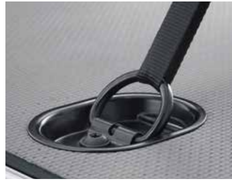
Load securing rings in load compartment floor. Can be used in combination with the optionally available tensioning straps to restrain the cargo.
