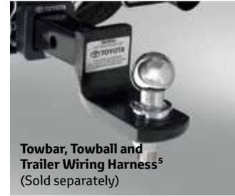
**Towbar, Towball and Trailer Wiring Harness<sup>5</sup>**
