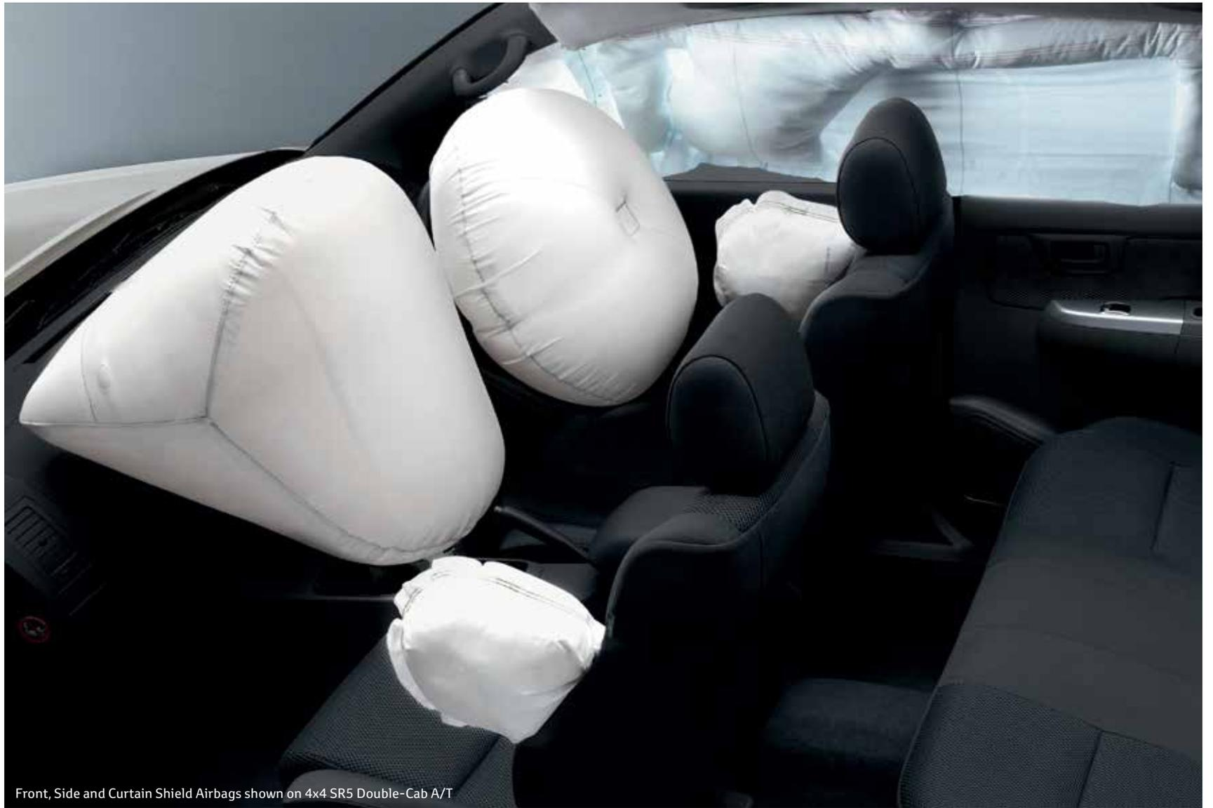
Front, Side and Curtain Shield Airbags shown on 4x4 SR5 Double-Cab A/T
