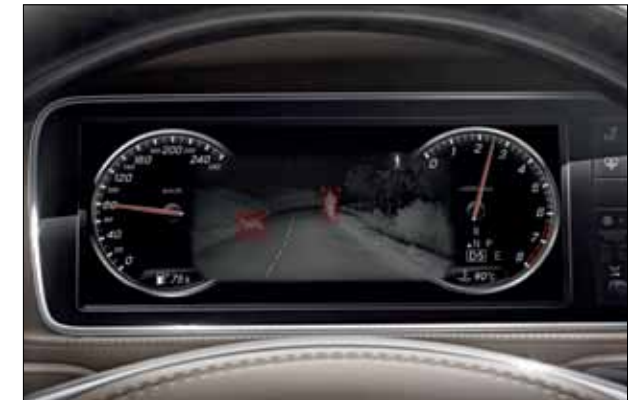
Night View Assist Plus highlights any people it has recognised and helps the driver to react quicker to dangers by night.
