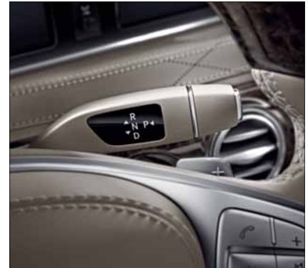
DIRECT SELECT lever on steering column. The driver can also change up or down a gear manually using the additional shift paddles.
