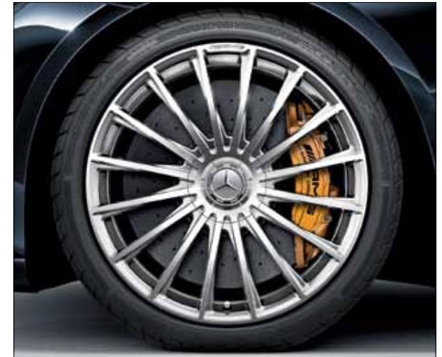
The standard-fit AMG 20-inch multi-spoke forged wheels with optional AMG ceramic high-performance composite braking system.
