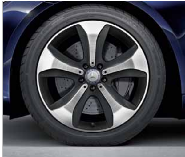
19-inch 5-spoke light-alloy wheels with 245/45 R 19 front tyres and 275/40 R 19 rear tyres.
