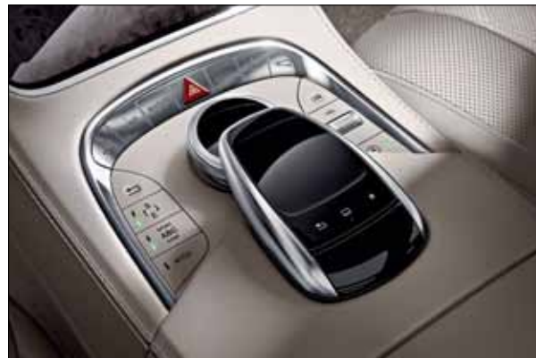
The touchpad allows convenient control of telematics functions using one or two fingers.
