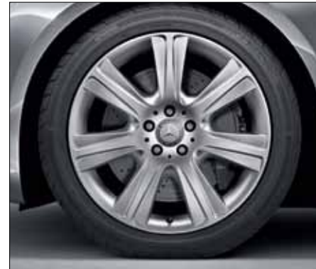
7-triple-spoke light-alloy wheels, painted in vanadium silver, with 245/45 R 19 front tyres and 275/40 R 19 rear tyres (Code 12R).
