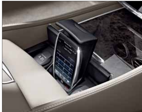
The optional handset with touchscreen serves both as a telephone and as a remote control for the seat functions of the optional Rear Seat Comfort package.
