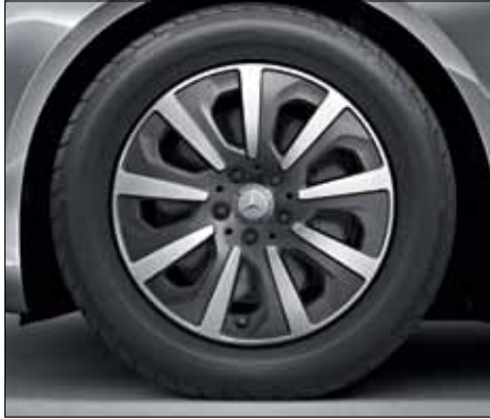
9-spoke light-alloy wheels, painted in tremolite metallic with a high-sheen finish, with 245/55 R 17 tyres (Code 09R).
