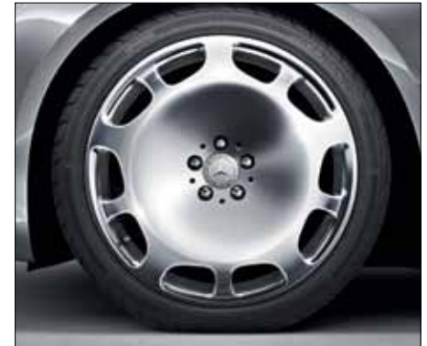
Forged wheels, painted in iridium silver, with 245/40 R 20 front tyres and 275/35 R 20 rear tyres (for Mercedes-Maybach only, Code 67R).
