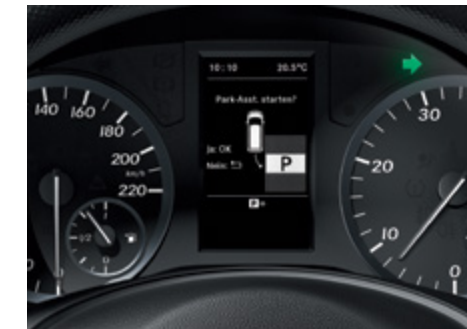
Active Parking Assist helps the driver find somewhere to park and assists when reversing into or out of a parking space.
