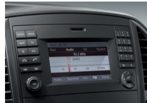
Audio 15 features a high-resolution 14.7 cm (5.8-inch) TFT display and numerous connection options.
