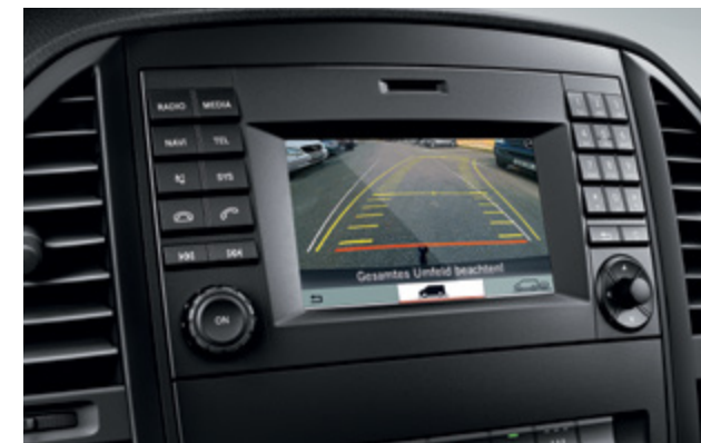
Reversing camera. The reversing camera is automatically activated when reverse gear is engaged. It assists the driver when reversing into a parking space. Static and dynamic guide lines show the driver the steering angle and the available clearance.
