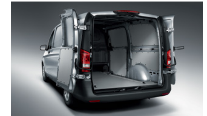
The two rear doors can be opened back to the side walls and secured, making loading and unloading easier. Optional equipment shown.
