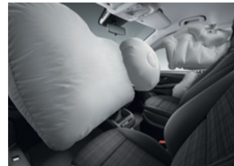
The airbags for driver and co-driver form part of the extensive range of standard-fit safety equipment. The optional thorax-pelvis sidebags and windowbags in the front offer additional protection.
