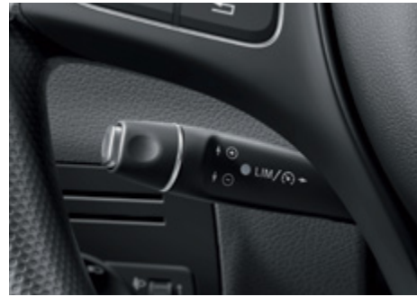
Cruise control helps to maintain a set speed, making the driver's job easier. *Overseas model shown.
