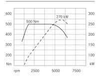
Engine speed rpm Torque in Nm
