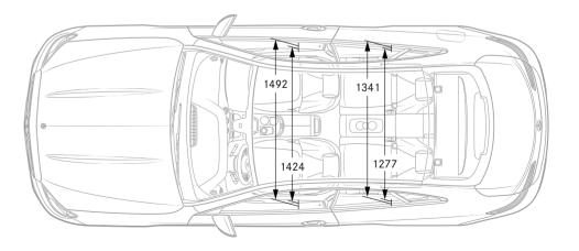
All figu es in millimetres. The illustrated dimensions are mean values. They are valid for vehicles in basic specification and in unladen condition
