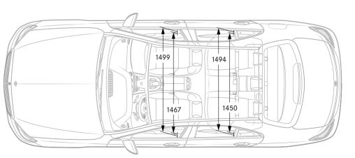
All figures in millimetres. The illustrated dimensions are average values. They are valid for vehicles in basic specification and in unladen condition.
