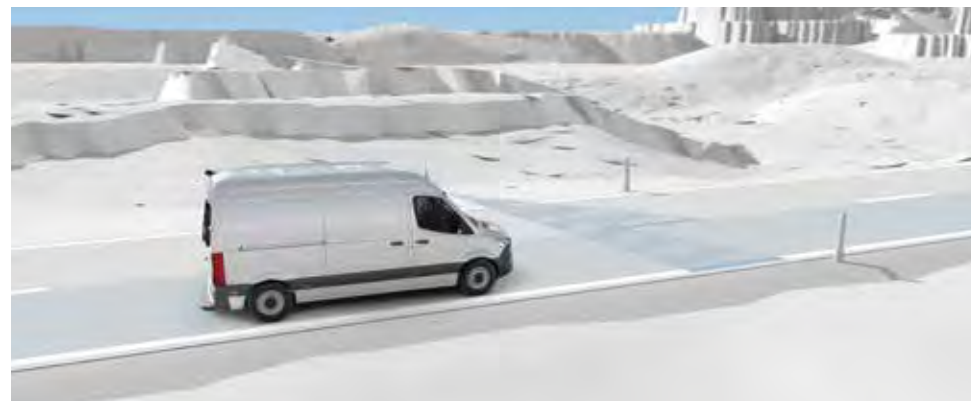
Active Lane Keeping Assist can help to detect when the vehicle is unintentionally leaving its lane, warn the driver and, if necessary, actively help to return the vehicle to its lane by means of braking intervention.
