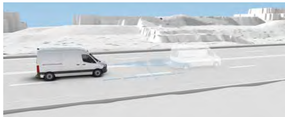
Active Distance Assist DISTRONIC can maintain the distance from the vehicle ahead as set by the driver and takes the strain off the driver in motorway driving or in stop-and-go traffic, for example.
