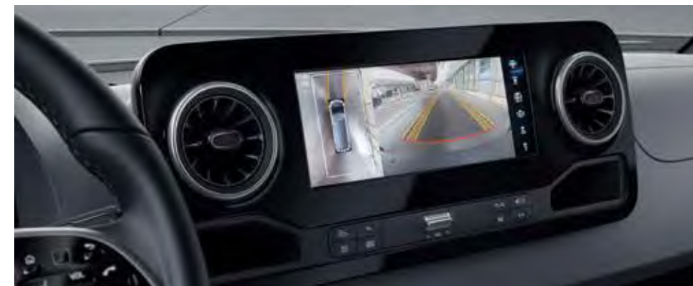
The Parking package with 360° camera provides comprehensive support when parking and manoeuvring, thereby enhancing safety and comfort.
