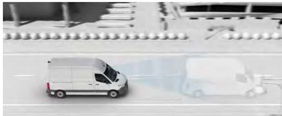
Active Brake Assist can help to avoid accidents with vehicle and crossing pedestrians ahead, or mitigate the effects of an accident.
