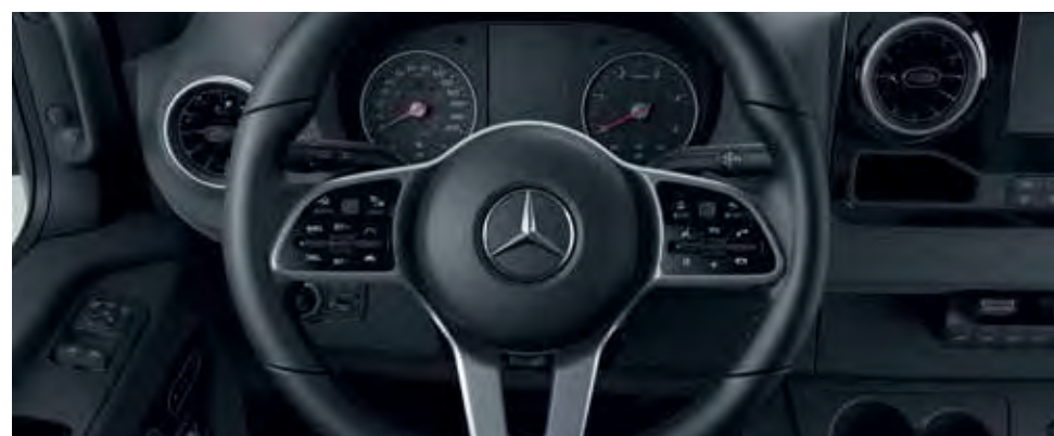
The multifunction steering wheel offers a convenient means of operating the on-board computer, vehicle functions and the multimedia systems via touch control or steering wheel buttons, without the driver having to remove their hands from the wheel.
