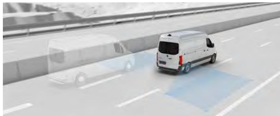
Blind Spot Assist with Rear Cross Traffic Alert can output visual and audible signals to help prevent accidents during lane changing, when reversing out of parking spaces and when dismounting the vehicle.
