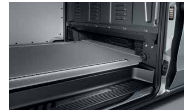
The driver and co-driver seats' open-backed seat base offers additional space for longer loads. Optional wooden floor.
