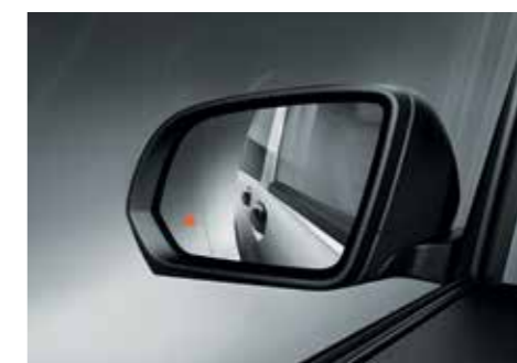
Blind Spot Assist can reduce the risk of accidents when changing lane, for example on freeways.
