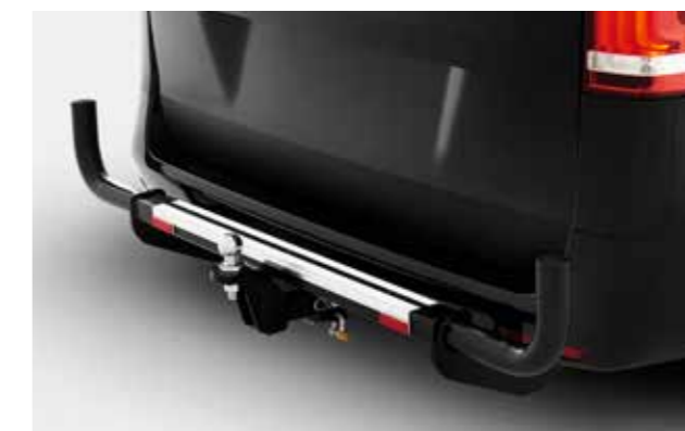
Rear Steps with rear lamp protection (with or without towbar). With a dual purpose this installation provides a sturdy step on the back of the van with the added bonus of rear lamp protection. Available with or without towbar.
