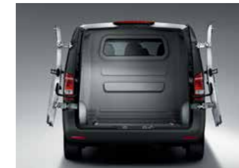
The two rear doors can be opened back to the side walls and secured, making loading and unloading easier.
