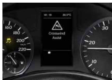
The Crosswind Assist function helps to reduce lateral displacement in the event of gusting side winds.
