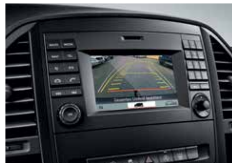
The reversing camera shows a photorealistic image of your surroundings with dynamic guide lines and an indication of the direction of travel. Excludes 111 models.
