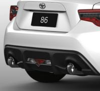
Dual exhaust tail pipes with diffuser
