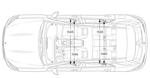
¹ At minimum to maximum height with steel suspension. All figures in millimetres. The illustrated dimensions are mean values. They are valid for vehicles in basic specification and in unladen condition.
