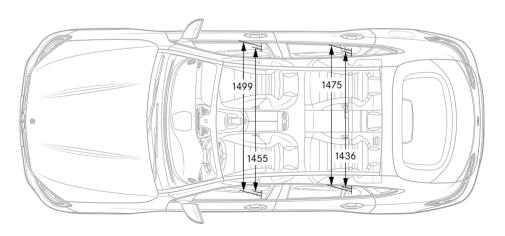
All figures in millimetres. The illustrated dimensions are mean values. They are valid for vehicles in basic specification and in unladen condition.
