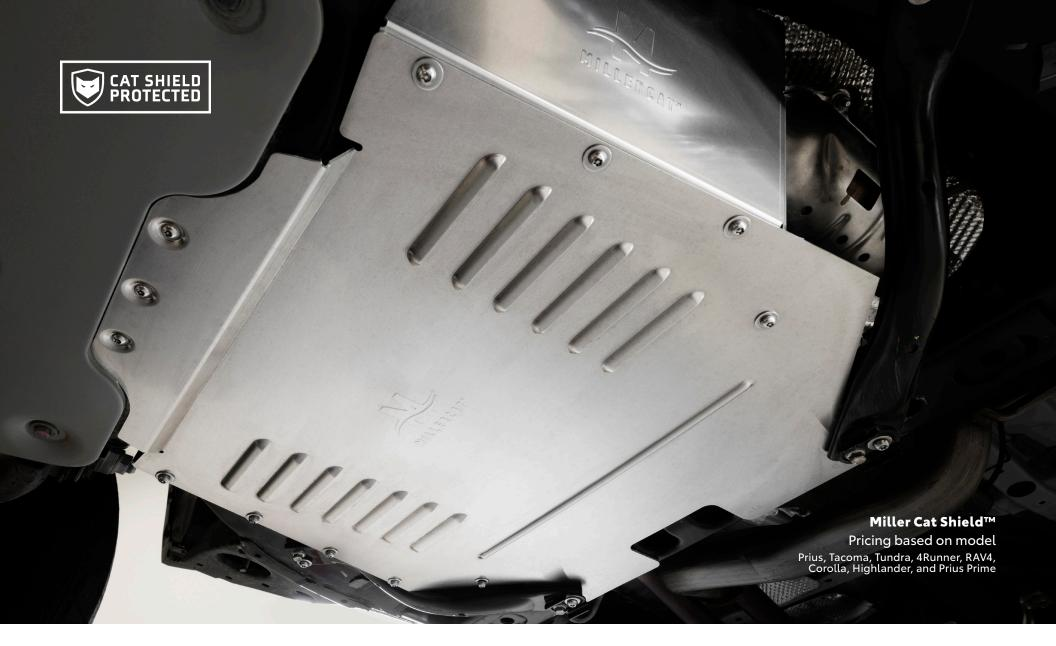
Miller Cat Shields are carefully crafted in stainless steel or aluminum to create a barrier to help protect the vehicle's most vulnerable areas from catalytic converter theft.
