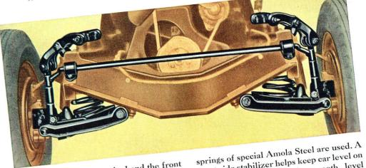
Road shocks are absorbed and the front wheels literally step over obstructions with DeSoto's independent front wheel springing. Extremely flexible and long-lasting coil
