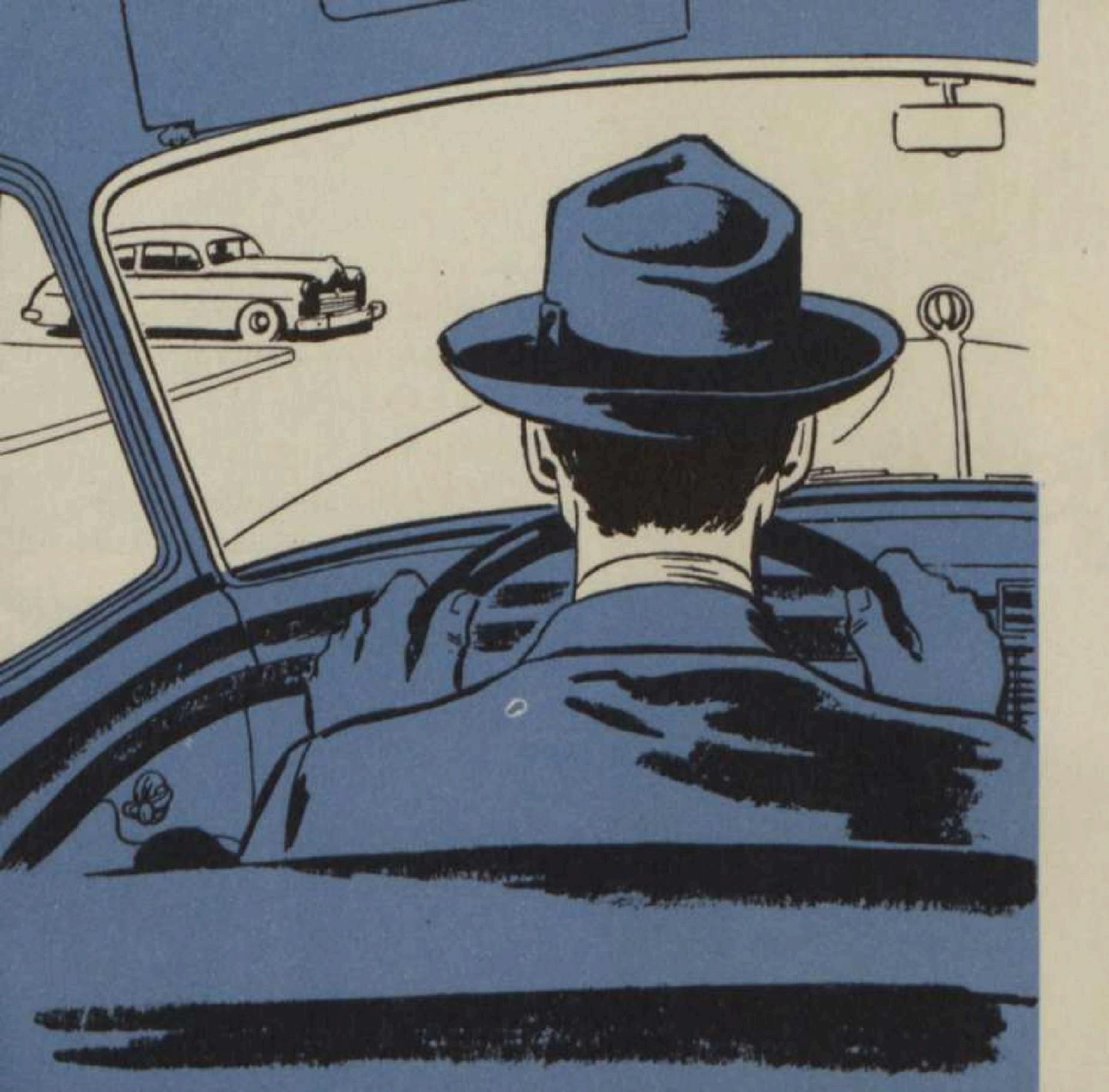
All windshields are curved in the 1950 Buicks. This results in corner posts being placed farther back.
