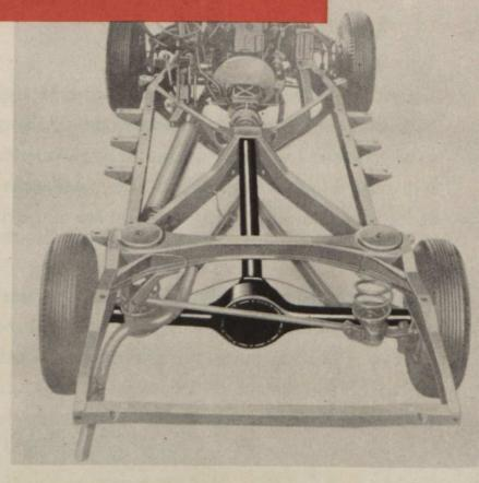
The solid "feel" of Buick is a characteristic quickly noticed after traveling in other cars. It comes from such structural features as this husky, X-braced frame and the torque-tube surrounding the drive-shaft.
