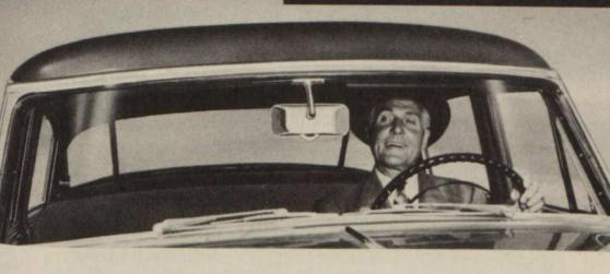
Wide-angle visibility is a feature of all 1950 Buicks, with their broad, high, curving windshields and narrow corner posts set farther back. Looking forward, you can see the road as much as 26 feet closer than in previous models. Overhead stop lights are easier to see, and cornering vision—such as when approaching side-streets—is noticeably better.
