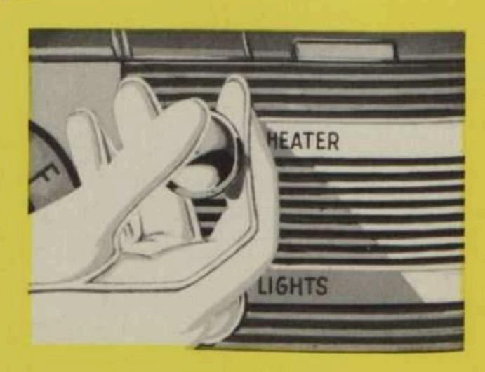
Pull this switch—marked "Heater" (3)—for floor-level heating of car. Now you have two-level heating, with uniform warmth in all areas of the car's interior. NOTE: Be sure to keep ventipane open slightly to insure proper circulation.
