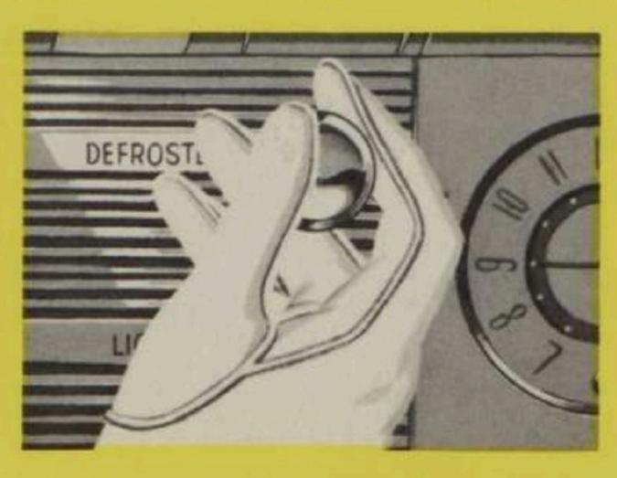
Pull this knob—marked "Defroster" (2)—to send warmed air through the car's upper level. Turn it to the right to switch on Blower—for forced draft of warmed air through upper level at slow speeds, or when car is stopped.
