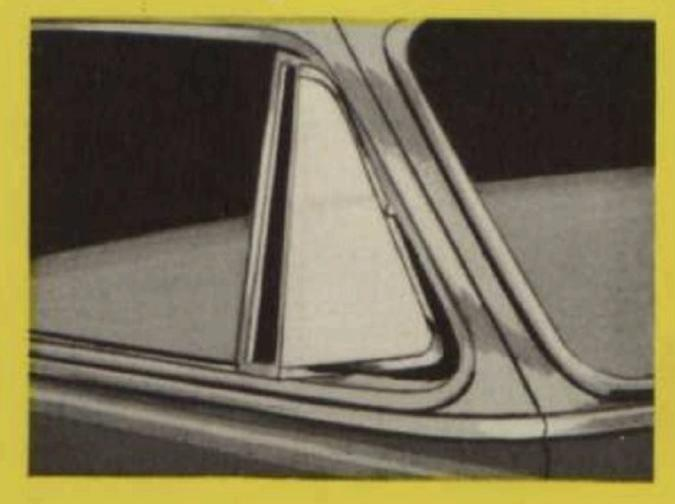
For complete circulation, keep ventipanes open slightly to insure constant flow of air through the car, even when it's raining and windows are normally closed.
