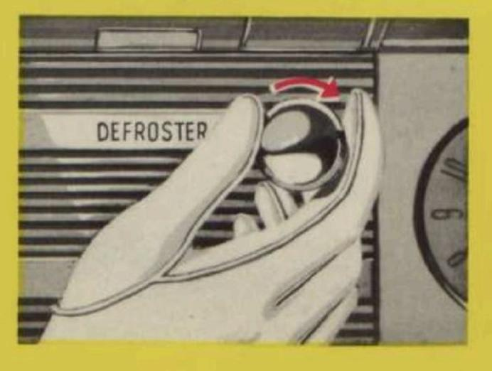
For upper-level ventilation, on both driver and passenger sides, push in "Ventilation" knob (5) and pull out "Defroster" knob (2). In the warmest of weather, while car is motionless or at slow speed, turn "Defroster" knob (2) to right to switch on Blower and forceflow a constant stream of outside air throughout the car.
