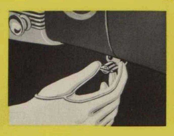
Set this thermostat control (1)—marked "Warmer"—for the temperature you want. Turn clockwise for higher temperature, counter-clockwise for lower, or "off." Temperature you set is kept even and constant, automatically—as in your own home.
