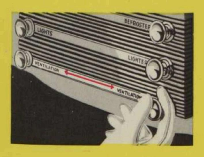
Naturally, you make sure thermostat control (1) is at full "off." Then you pull out "Ventilation" knobs (4 and 5) on left and right sides to direct large volume of outside air to lower level of driver and passenger side respectively—and independently. Notice how this air circulates under the front seat to cool and refresh the rear seat passengers.
