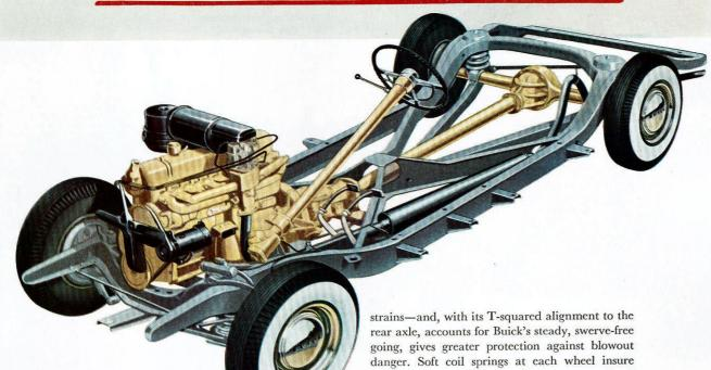
This is the ready-for-anything chassis that makes the SPECIAL'S going so true and steady. Note the massive X-braced frame for balanced rigidity. The full-length torque tube takes all driving thrust, frees rear springs of driving
