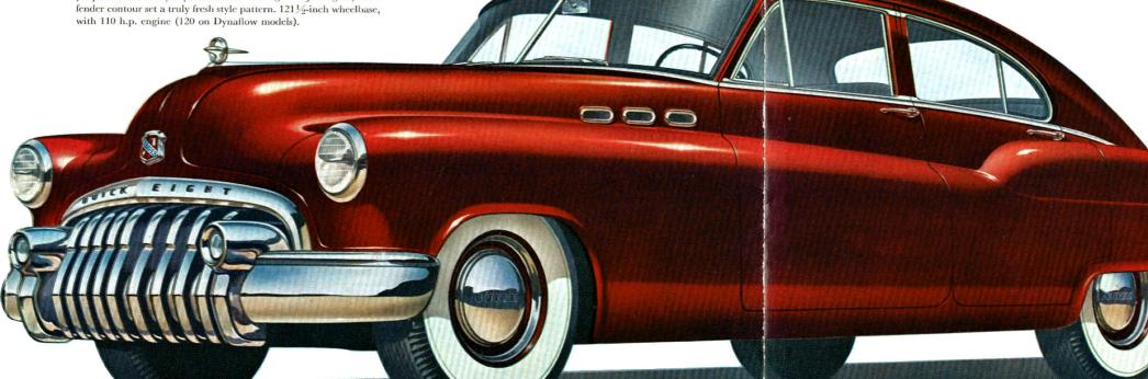
DOUBLE-DUTY BEAUTY-Better to look at, and nonlocking, too-that's the SPECIAL idea in joining gleaming grille with massive bumper. Grille bars are additional bumper guards, as strong as those which mount the combined parking lights and direction signals.
