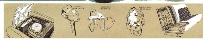
New counterbalanced, front-hinged hood means easier servicing—safer, too. Ford's new 2-stage door checks hold the big front doors open in
