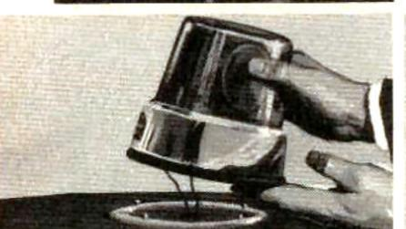
ROOF LIGHT WIRING FOR FLASH-ER. 5 color-coded wires, easily accessible for local installation. (They are temporarily attached to domelight fixture). No hole in roof.
