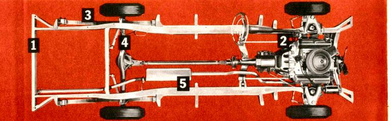
HEAVY DUTY SAFETY POWER CHASSIS. Full-length side rails of heavy girder steel, box construction, give officers protection in side collisions—unlike X type frames. Live rubber body mounts completely eliminate metal-to-metal contact between body and frame. Additional rigidity comes from massive cross-member which supports engine and front suspension.
