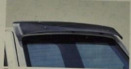
The rear air deflector for the Multi is designed to improve the aerodynamics of your vehicle while keeping the rear window free of dirt and dust for safety and visibility.
