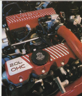
Right: The 2.0 litre turbo engine has 165 horsepower.
