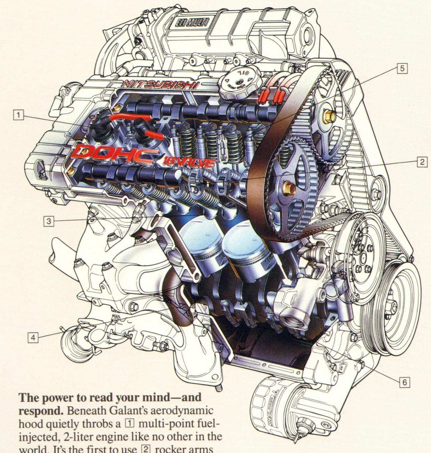
world. It's the first to use 2 rocker arms with needle roller bearings, a Mitsubishi exclusive that greatly reduces friction loss in the valve train. Result: a smooth-running high-revving powerplant that starts fast and responds even faster.
