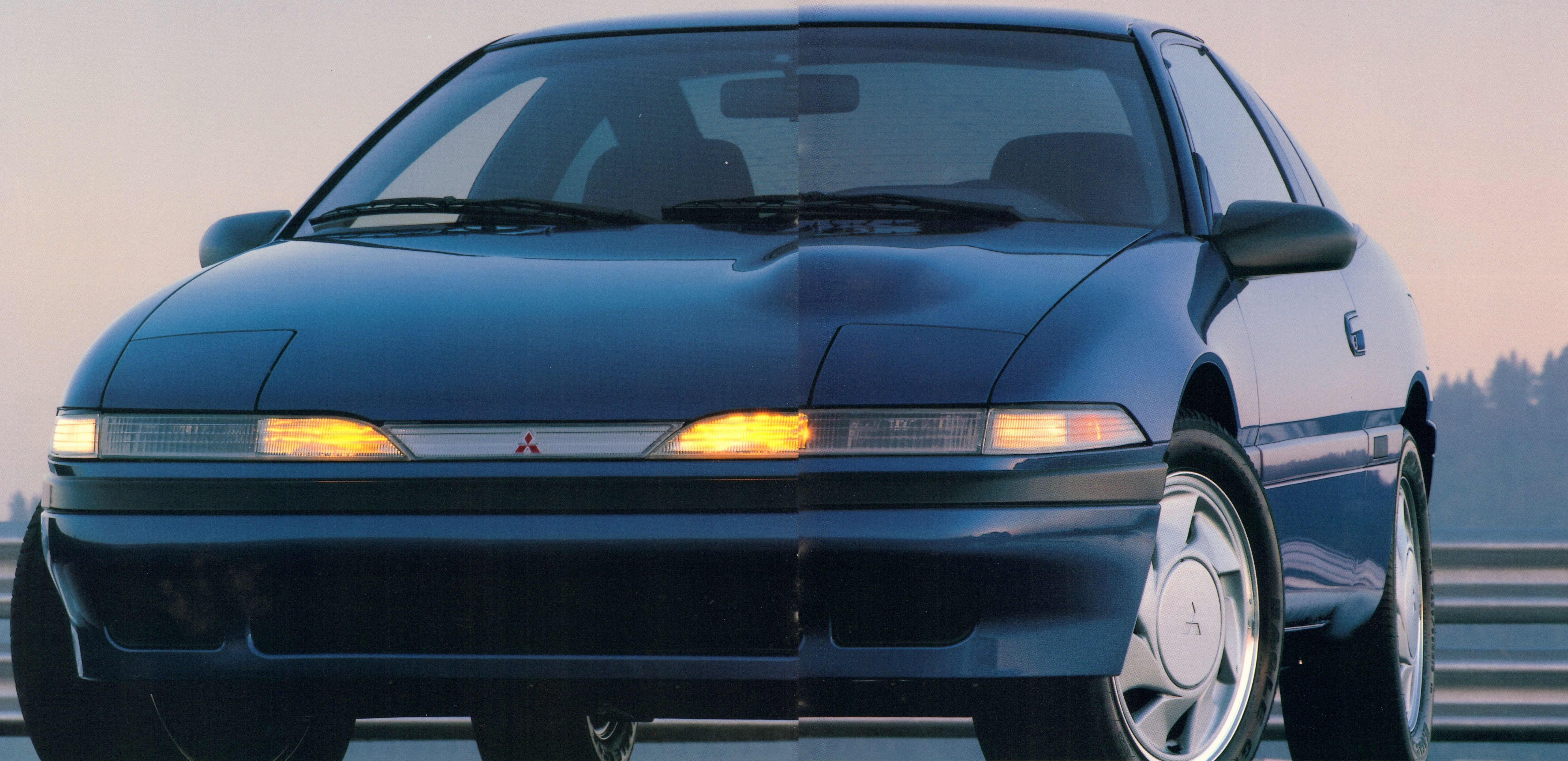
Eclipse GS DOHC 16-Valve responds with 135 horsepower at 6,000 rpm.
