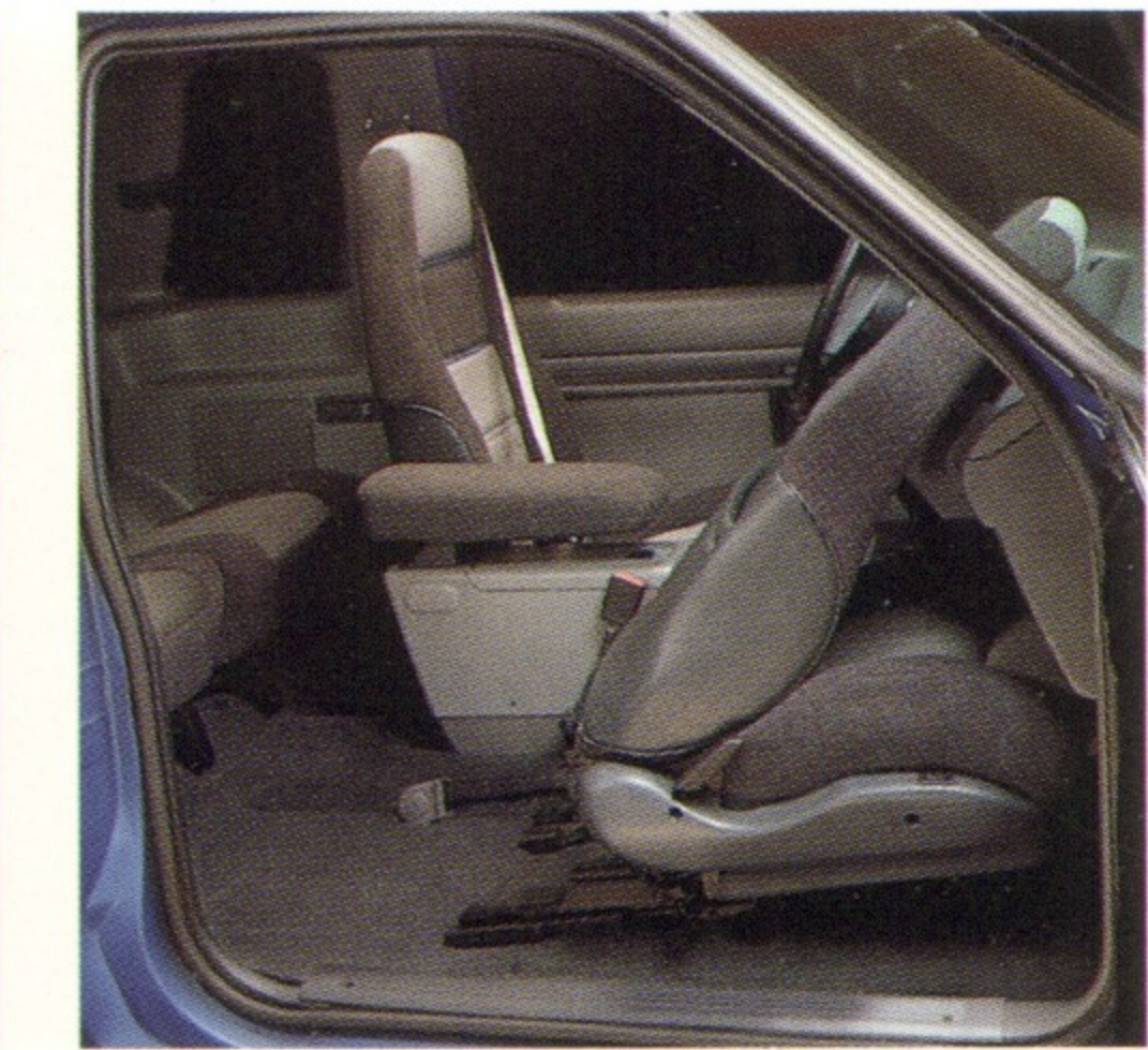
"Tip-and-slide" front bucket seats slide out of the way at the touch of a lever, making it easy to get into or out of the rear seat. The entire operation can be accomplished with just one hand.
