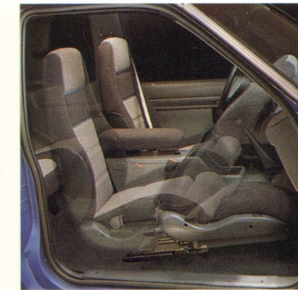
"Tip-and-slide" front bucket seats slide out of the way at the touch of a lever, making it easy to get into or out of the rear seat. The entire operation can be accomplished with just one hand.
