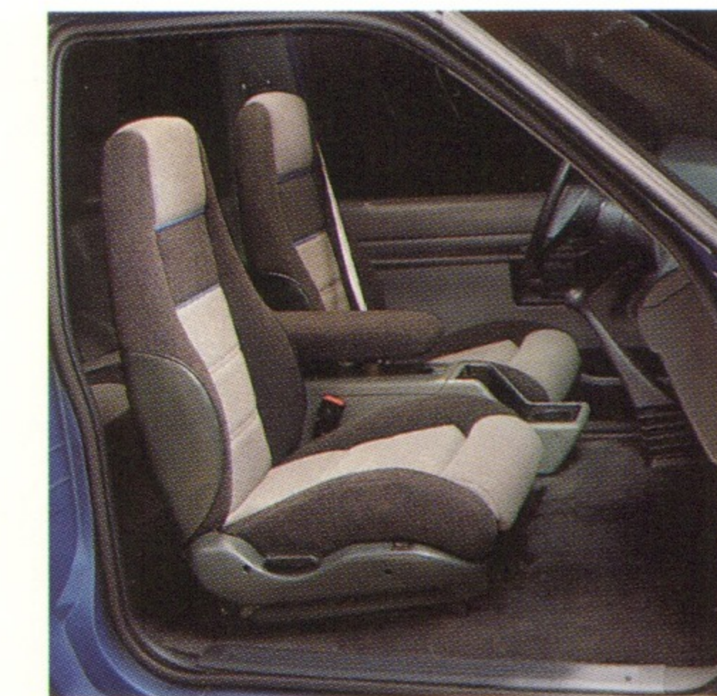
"Tip-and-slide" front bucket seats slide out of the way at the touch of a lever, making it easy to get into or out of the rear seat. The entire operation can be accomplished with just one hand.
