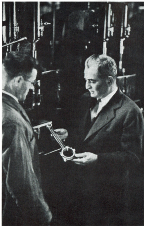
Diamonds are actually worn out in drilling to a jewel-like smoothness such quality parts as the bearing surfaces of the connecting rod which Mr. Roberts is inspecting.
