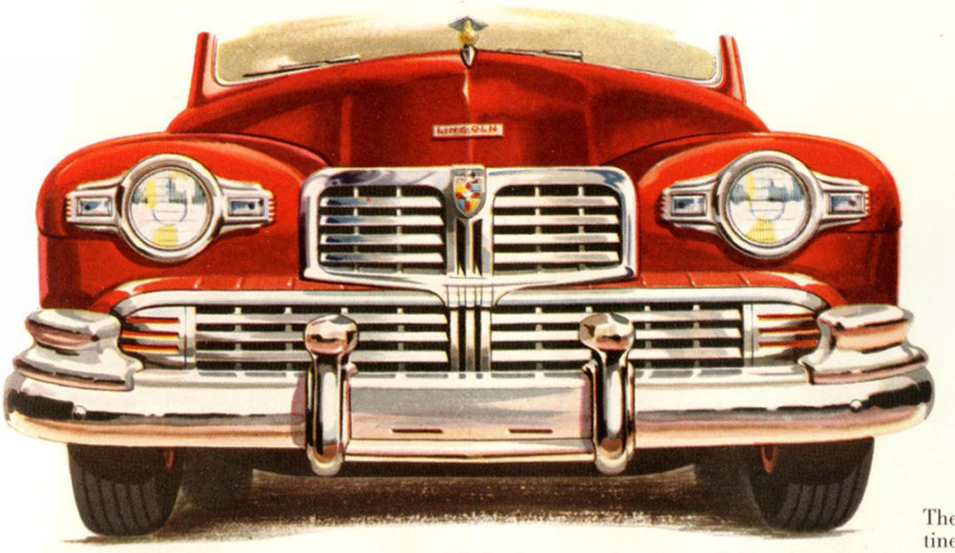
All the beauty and artistry of the original design have been perfectly executed in the new segmented grille. When installed, auxiliary road lamps set flush with the grille.
