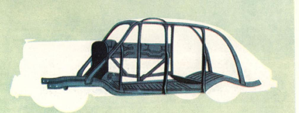
The welding of the top and side panels with the truss-type assembly forms a unit body frame of exceptional strength in relation to its weight. This results in a unit structure highly resistant to twisting or flexing.
