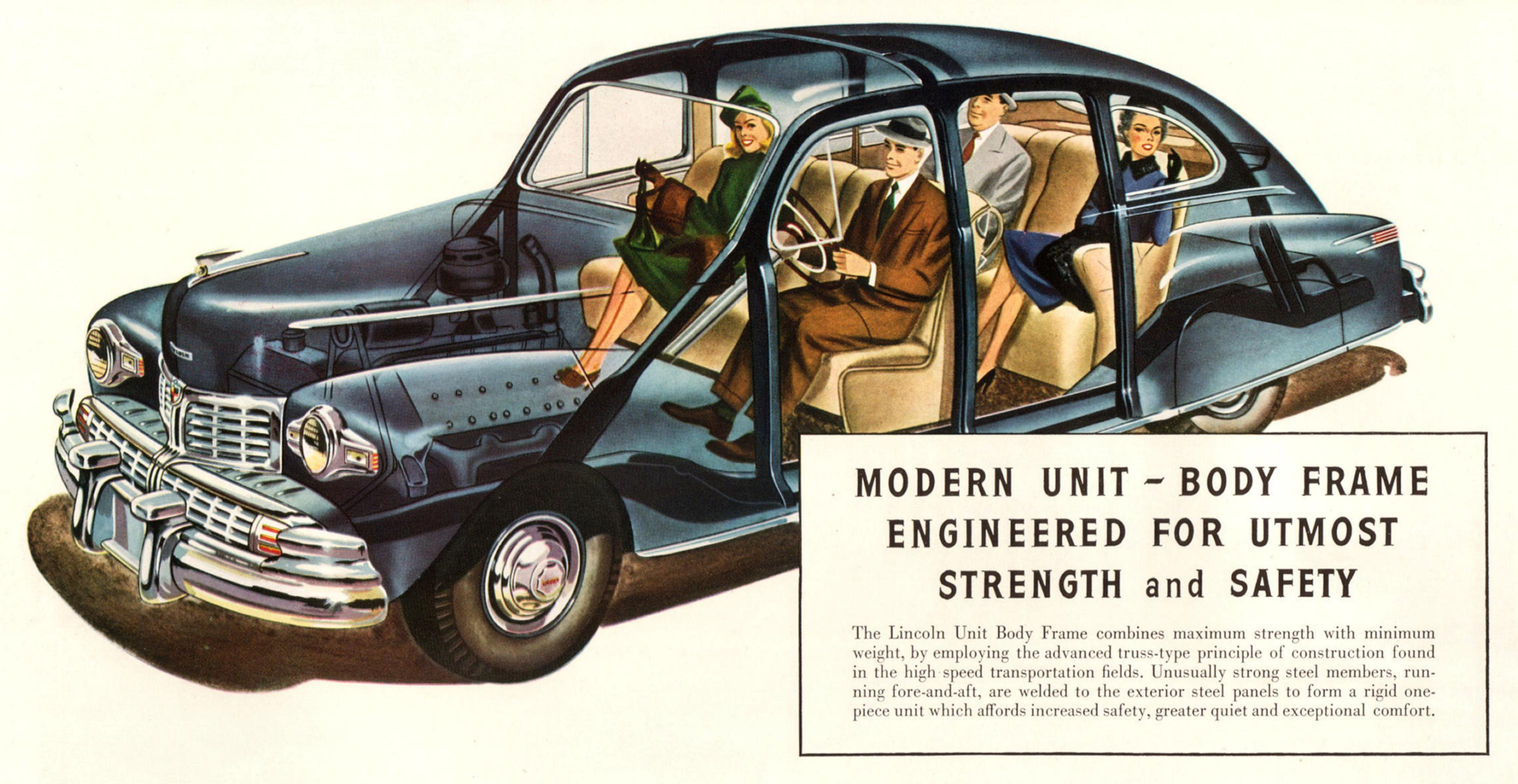
The truss-type structure is achieved by welding strong internal members to the sturdy steel floor. Note the diagonal steel reinforcements which run forward from the base of the windshield.
