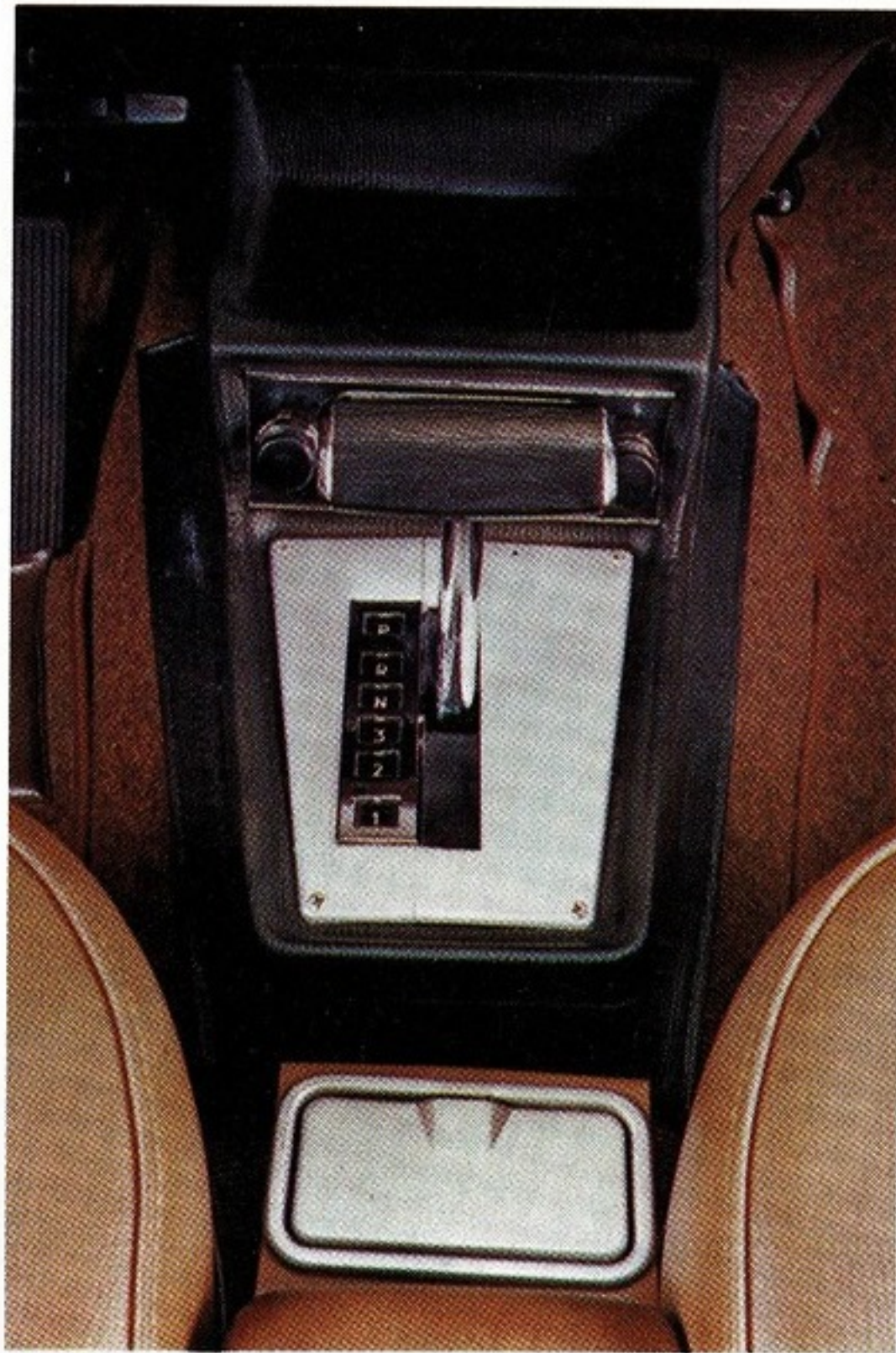
Optional ZF automatic transmission (Standard transmission stick shift is floor mounted)
