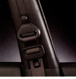
EMBRACE. Camry Sedans and Wagons come equipped with adjustable front shoulder belt anchors that enhance driver and front-passenger comfort. Passenger seats feature an Automatic Locking Retractor (ALR) that locks for child safety seats.
