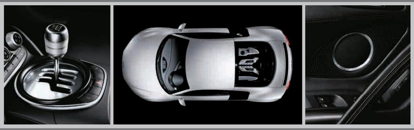
**Transmission**: Standard six-speed manual transmission. Optional R tronic<sup>™</sup> – a direct-shift, six-speed gearbox with shift-by-wire technology. Complete with paddle shifters as well as a joystick gear lever. Combines the sportiness of a manual gearbox with the advantages of an automatic.
