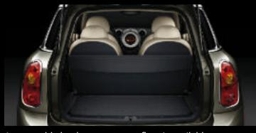
A removable load compartment floor is available as an option to cover the storage-well.
