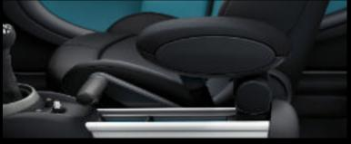
The available center armrest adjusts into three positions and includes a dish for storage.
