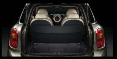
The standard floor of the luggage compartment can be folded up to separate the luggage area from the passenger space. When it is folded down, it covers the storage-well.
