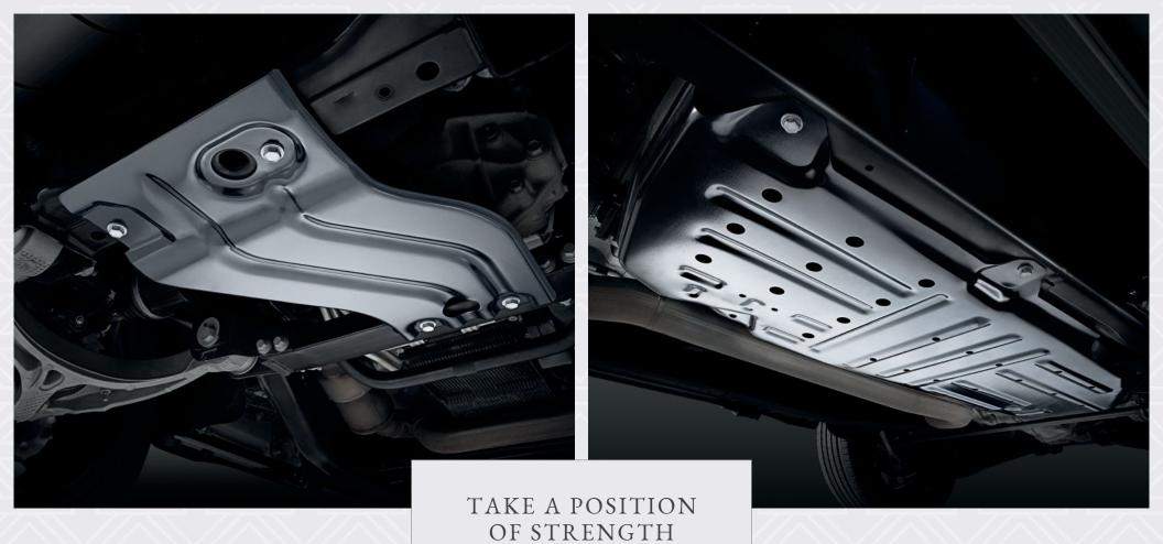
SKID PLATES — Heavy-duty steel plates, painted with a high-quality black powder-coat finish, offer serious underbody protection when covering rough terrain. Available for the Front Axle, Fuel Tank and Transfer Case.
