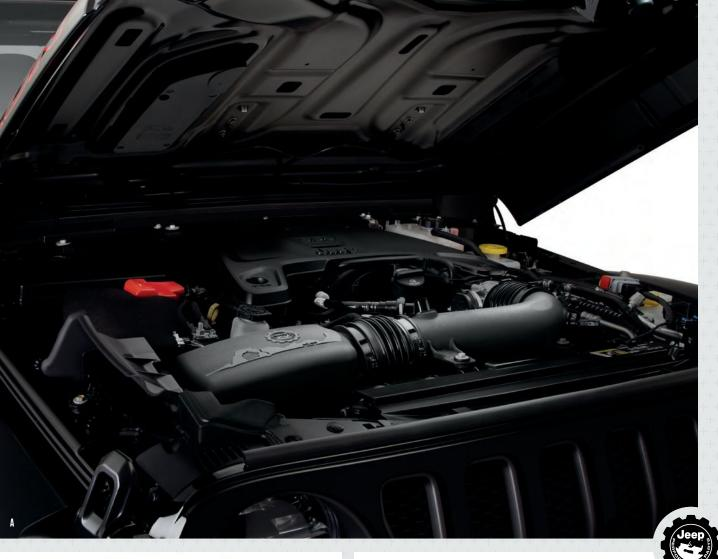
A. COLD AIR INTAKE SYSTEM. Features Jeep Performance Parts logo and reusable black and silver drop-in filter. Draws fresh air from outside vehicle into hood cutout to increase engine performance. Available for 3.6L engines only and includes bezel to finish cutout. [77072433AC]
