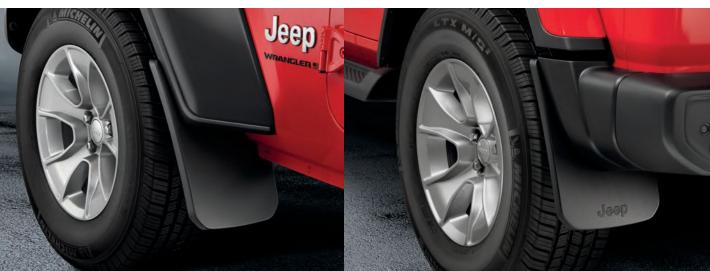
MOLDED SPLASH GUARDS. Designed to provide excellent lower-body protection by minimizing the spray of water, mud, snow and rocks. Fit front and rear wheel wells of the Jeep<sub>®</sub> Wrangler Sahara<sup>®</sup> or Sport. Front Splash Guards do not fit vehicles equipped with Rock Rails.
