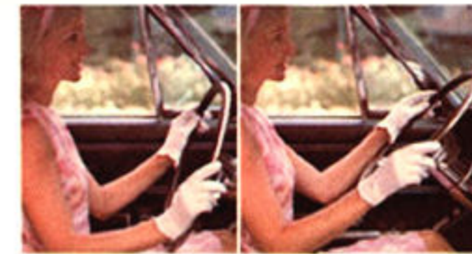
Tilt steering wheel. No need to adjust yourself to the steering wheel when you can adjust the steering wheel to yourself. Buick's adjustable steering wheel locks into any one of seven positions, to fit everyone from the tallest to the smallest. Flip it up out of the way, too, to make getting in and out easier. Available on LeSabre, Wildcat, Electra 225 and Riviera.
