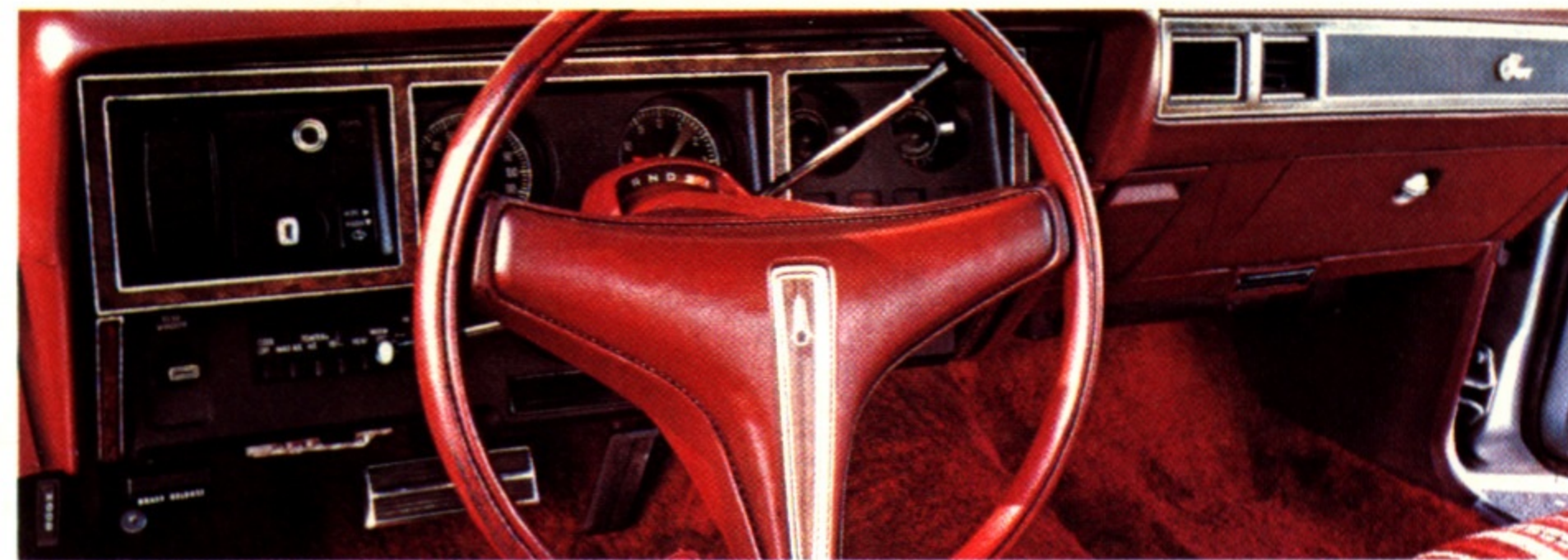
Newly styled, newly engineered instrument panel. All standard gauges, switches, heater controls can be removed at panel face for easy repair.
