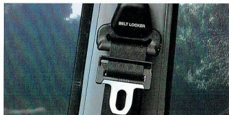
Belt-locker device prevents payout of seat belt webbing in extreme circumstances.
