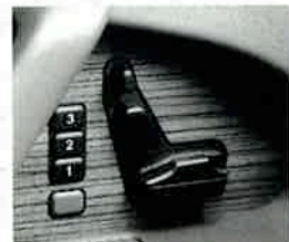
Front seats can be power-adjusted 12 ways with logical seat-shaped controls.
