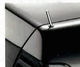
Pop-up reversing guides rise to assist in backing up, then silently disappear.
