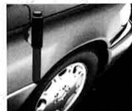
Adaptive Damping Suspension is driver adjustable for Sport or Comfort mode.
