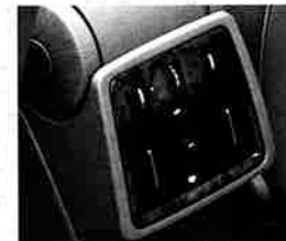
Rear compartment air conditioning has individual left and right controls.
