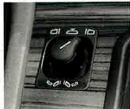
Position of electric inside and outside mirrors is included in the seat memory.
