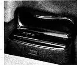
CD changer is concealed in the trunk and operated from the radio controls.
