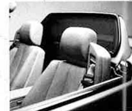
Wind deflector reduces noise and turbulence, can be stowed away in trunk.
