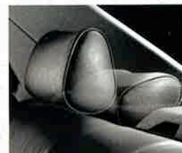
The driver can fold down the rear head restraints using a dashboard switch.
