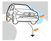
ESP brakes the outside front wheel to counteract oversteer.
